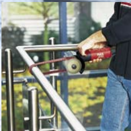
THIS ROUNDS IT OFF Rubber drive roller and polishing fleece mirror-finish stainless steel guard-rails. Burnishing machine LP 1503 VR PROFI kit ▶ on page 26
