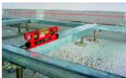
Laser water level with laser line e.g. for transferring heights.
